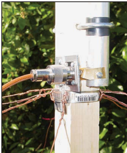
Figure 4—Radials are wrapped around a hose clamp and pressed against the antenna connector. A brass strap is soldered to the connector center conductor and then bolted to the vertical radiator. Two U bolts hold the vertical radiator to the mast.
