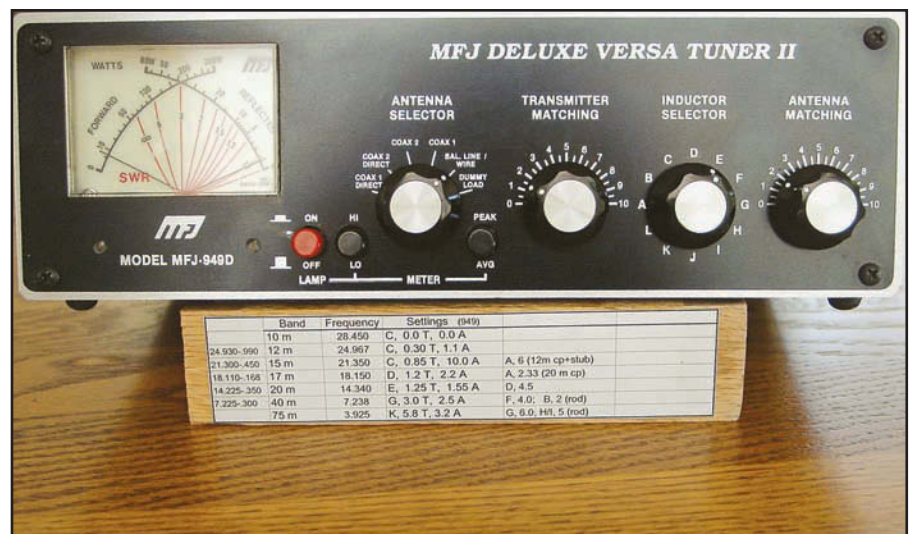
Figure 2—Antenna tuner settings can be recorded on a chart for faster band changes.
